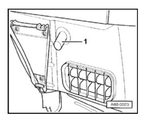
Rear water drain hoses are routed in the C-pillars and exit behind the bumper cover at the side. They can be cleaned from the lower end of the hose. To do so, rear bumper cover must be removed.
