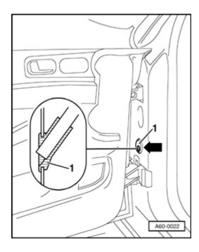
Front water drain hoses are routed in the A-pillars and exit above the lower hinge of front door.
